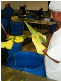
The outer leaf is tough and leathery and it takes a very sharp knife to top and tail the leaf and to cut off the sides in order to leave a gel sandwiched between the outer sides of the leaf. These pre-prepared fillets are placed into drums and then pass on through the factory to the next stage
